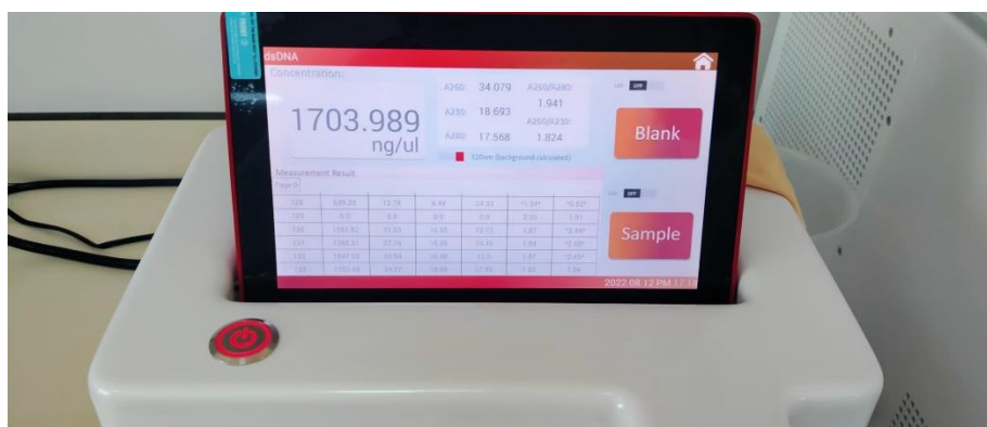
Figure 7: Quantification of DArTseq protocol isolated DNA of genotype 1 with Maestrogen MaestroNano Pro Spectrophotometer
