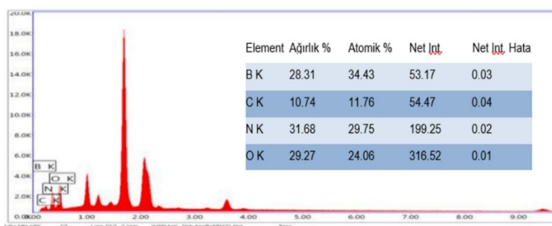
Figure 5. SEM-EDS analysis of hBNN(3:7).
