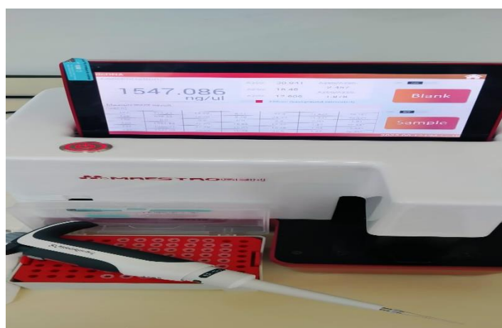
Figure 6: Quantification of CTAB protocol isolated DNA of genotype 1 with Maestrogen MaestroNano Pro Spectrophotometer
