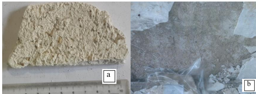
Figure 2. Back face of the sample (a), Location of the sample on the work (b)
